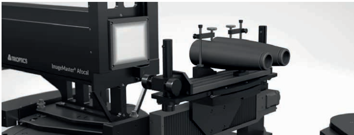
Illustration 2: Sample mounting of binoculars
