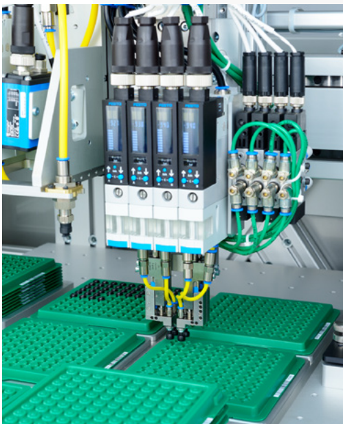
Pick and place of lenses by 4 gripper system
